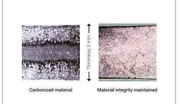
Figure 2 | Standard heat stabilized polyamide (left) vs. Radilon® A RV350HHR (right) after heat ageing at 210°C.
