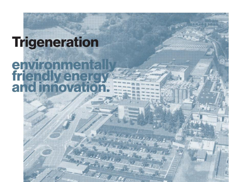
An innovative high-efficiency trigeneration plant at Radici Yarn, a plant in the RadiciGroup ATS area, was installed in 2019, and became fully operational in 2020. The plant, which runs on methane gas, is used for the simultaneous production of steam and electricity, typical cogeneration factors, plus the production of chilled water used for the industrial process.
